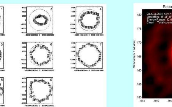
Visibility amplitude as a function of grid position angle, shown as polar plots for subcollimators with FWHM resolutions ranging from 2.3 to 183
