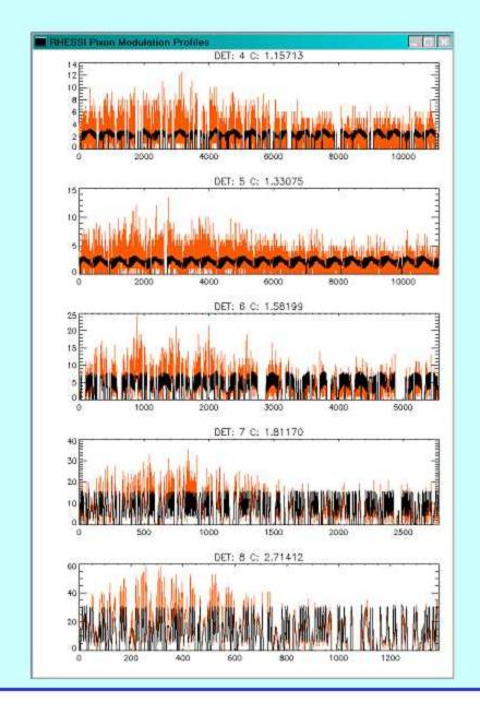
Stacking data using spacecraft roll angle and 'aspect phase' makes long data sets equivalent to a single rotation.
