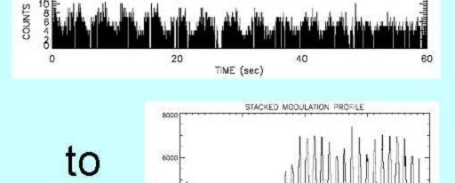
The same data summed into 288 roll/phase bins, shown as a linear raster in aspect phase, then roll angle.
