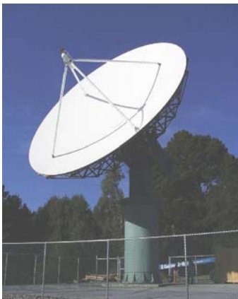
Figure 3. BGS 11-m antenna system located at UCB/SSL.
