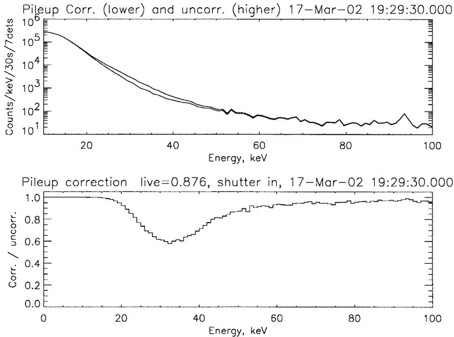
Figure 13. Pileup correction at modest deadtime with the thin shutter in place. *Top*: count spectra before and after pileup correction. *Bottom*: ratio of corrected to uncorrected spectrum as a function of energy.
