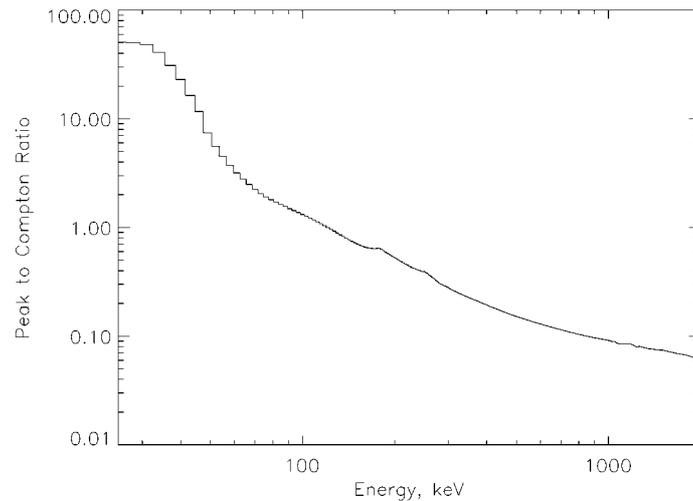
*Figure 11.* RHESSI response matrices: photopeak to Compton-continuum ratio versus energy. The continuum contains every simulated photon which leaves less than its full energy but more than 3 keV in the detectors.
