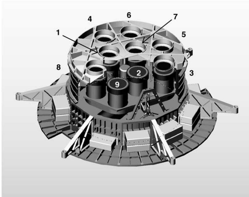
*Figure 4.* Exterior of the spectrometer shown with part of the outer housing cut away, revealing the detector modules inside. The numbering scheme of the detectors matches the grids.
