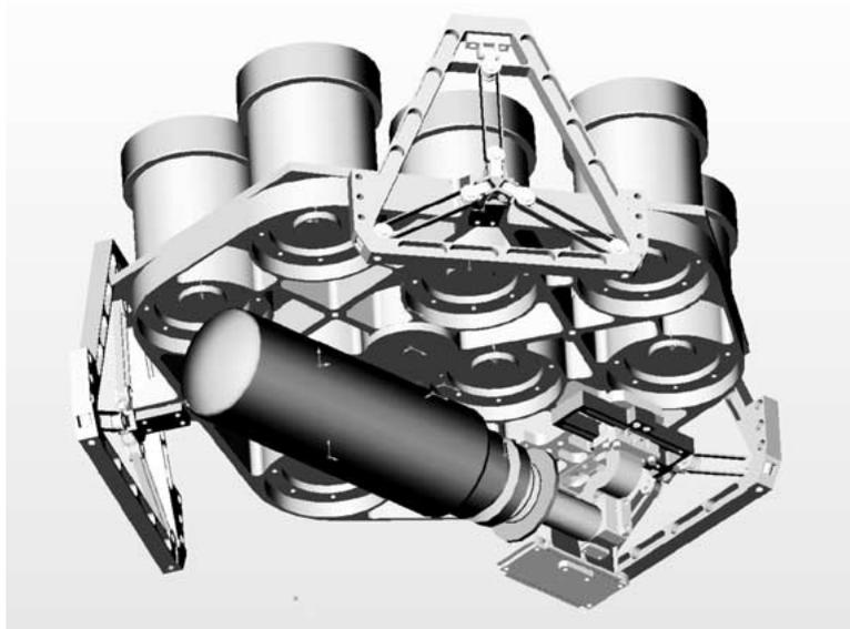
*Figure 5.* The interior of the RHESSI spectrometer, showing the detectors mounted on the coldplate, the Sunpower cryocooler below it, and the fiberglass-strap 'cartwheels' that suspend this assembly in the interior of the cryostat.
