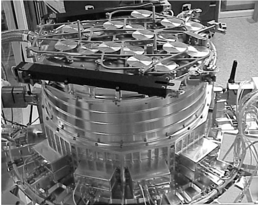
*Figure 3.* The RHESSI spectrometer, before being mounted on the spacecraft. The aluminum attenuator disks are visible on top (one set in the aperture, the other out), and the preamplifiers and high-voltage filter boxes can be seen around the skirt. The detectors are behind the thin, ribbed side wall.
