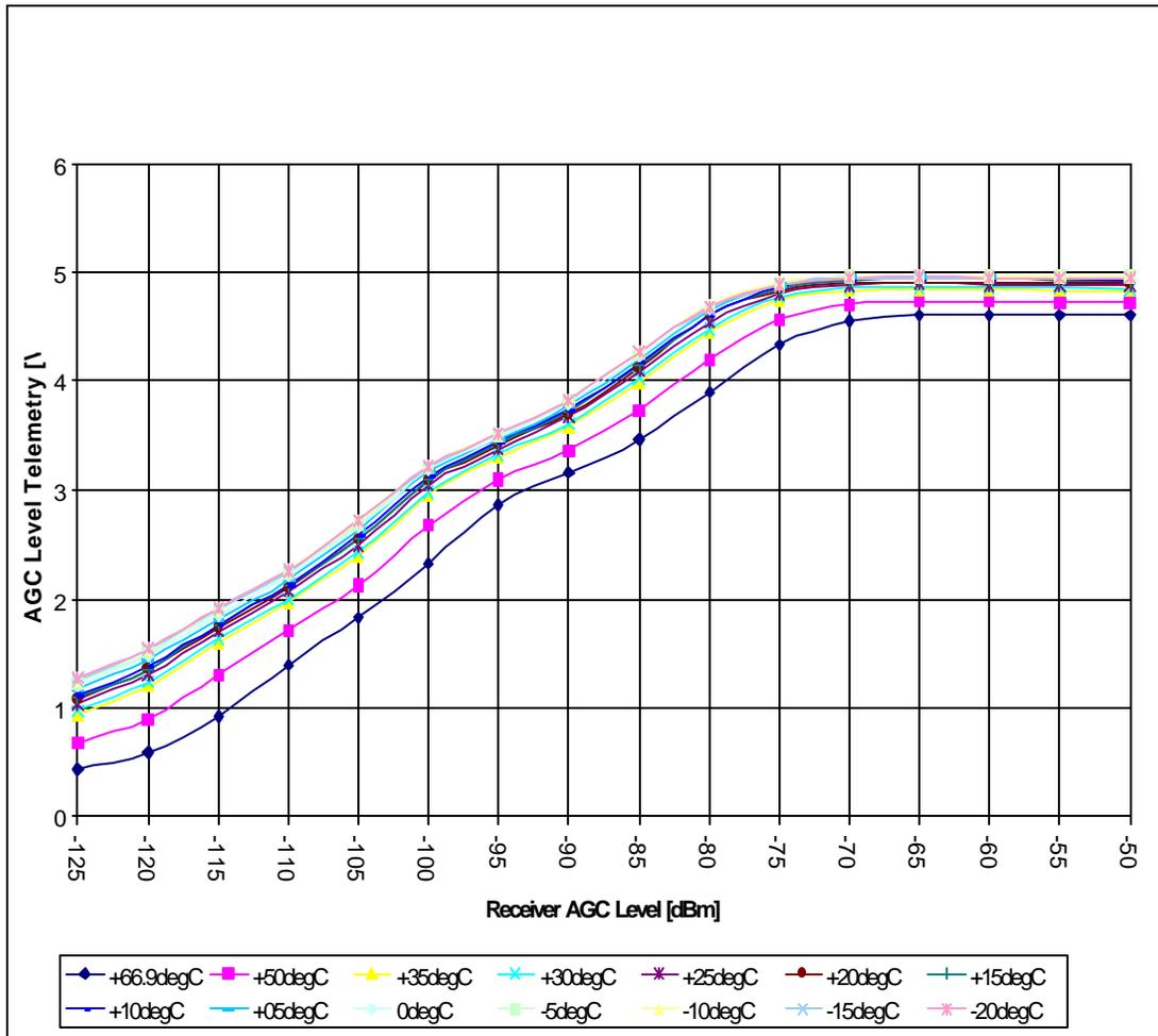
Figure 4: Conversion curves for the receiver AGC level telemetry.
