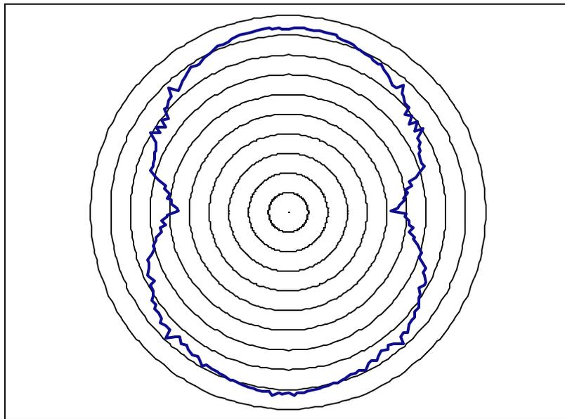
**Figure 5:** This figure shows the HESSI transmit antenna pattern. Gain circles are spaced by 5 dB, starting at +10 dBi with the outermost circle. The top half is the pattern of the forward transmit antenna, and the bottom half the pattern of the aft transmit antenna on the spacecraft. The spacecraft's spin axis points along an imaginary top-to-bottom line.
