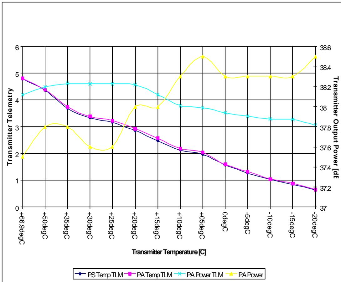
**Figure 2:** Transmitter temperature and output power telemetry.
