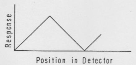
Figure 2. Principle of operation of a simple imaging modulation collimator. The lower grid has slightly smaller holes than the upper grid. The response as a function of position in the detector has the same triangle-wave nature as the time function in Figure 1. The angular resolution is the same (FWHM = d/D) but the position dispersion of the "image" may be varied by changing the grid parameters slightly.
