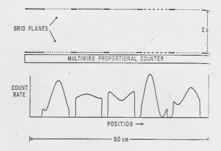
Figure 4. Schematically illustrates the count distribution in five subcollimators (see Fig. 3) with position-sensitive proportional-counter readout. Each subcollimator has different angular parameters and a different visibility.
