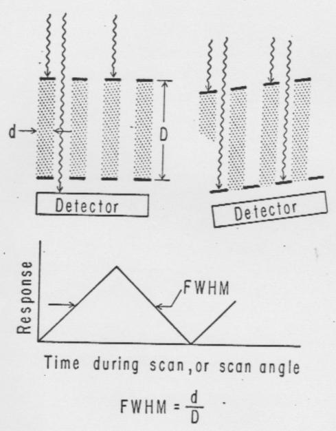
Figure 1. Principles of operation of the two-grid modulation collimator, showing how a point source produces a triangle-wave modulation of the counting rate as the collimator sweeps in angle. The angular resolution is determined by the ratio of hole size to collimator length.
