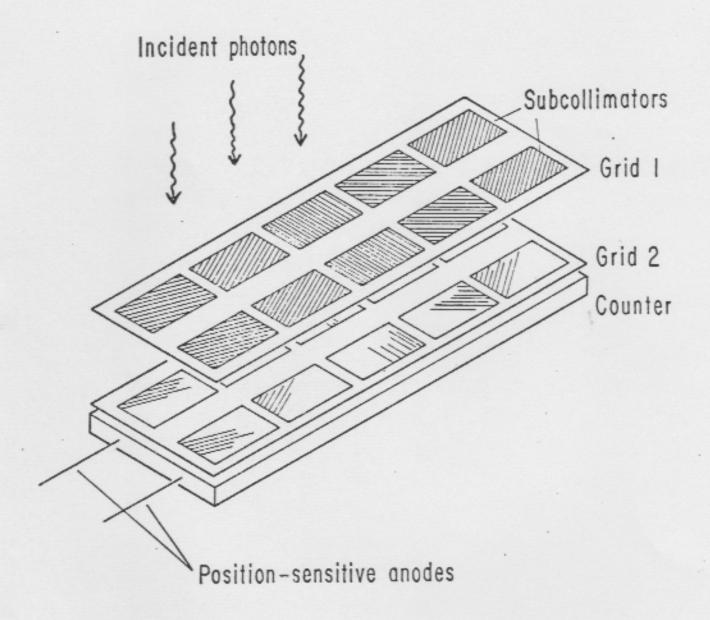
Figure 3. Sketch of layout for a two-grid imaging collimator and a position-sensitive proportional counter. The wire spacings differ (as illustrated in Figure 2) so that one Fourier component is distributed along the direction of position sensitivity. The slits do not need to have the same orientation as this direction: the sketch shows ten individual subcollimators or "baselines".
