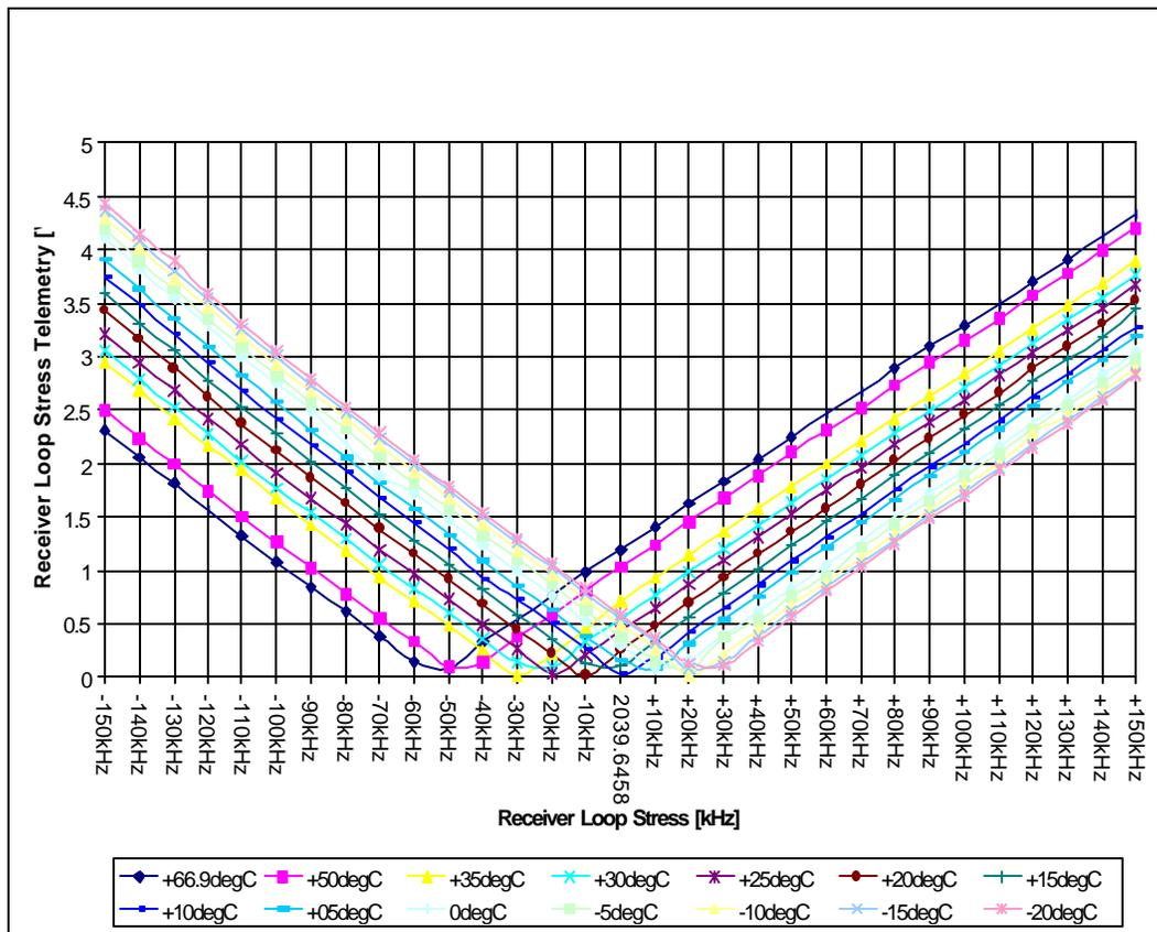
Figure 3: Loop stress of the RF phase-locked loop in the HESSI command receiver.
